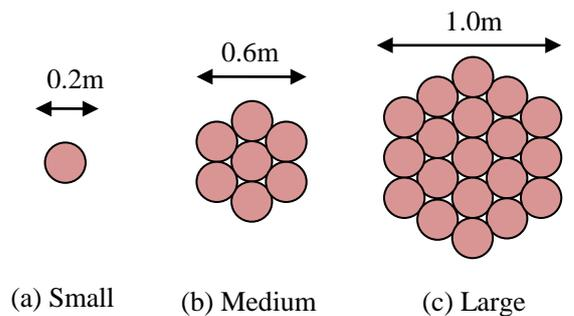
Figure 7 Size of rocks incorporated in the debris flow model
