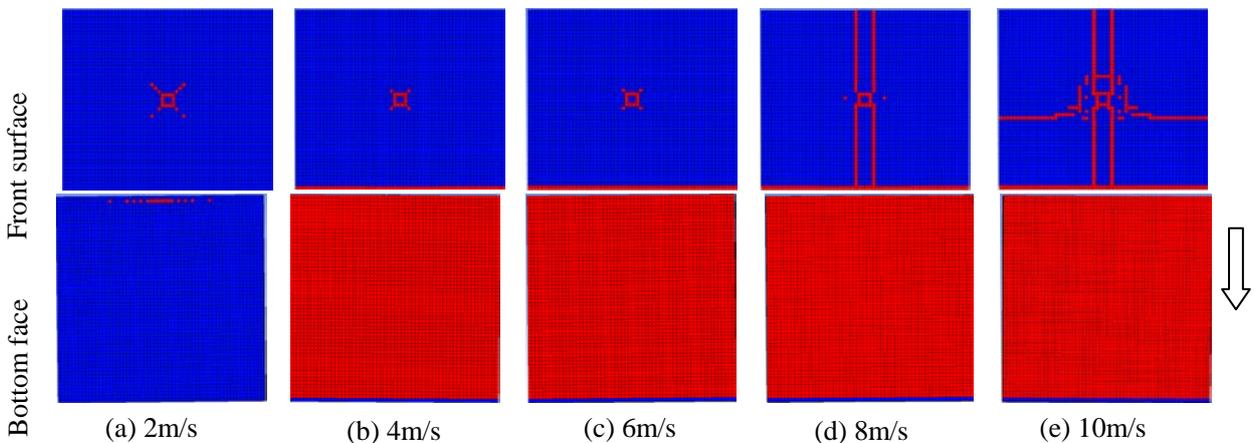
Figure 6 Failure states of concrete dam wing (Impacting rock diameter of 1m)
