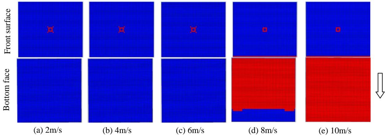
Figure 5 Failure states of concrete dam wing (Impacting rock diameter of 1m)
