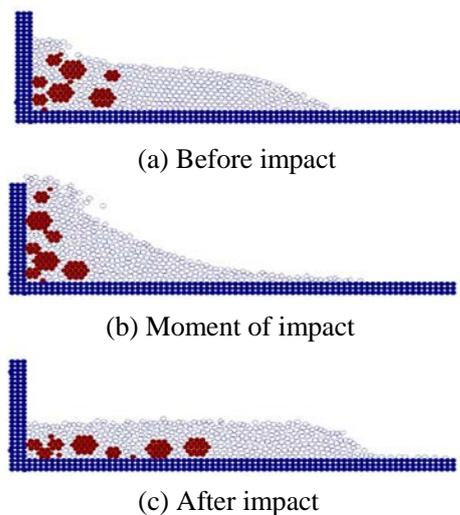
Figure 9 Impact of rocks included in the debris flow onto the dam's concrete wall
