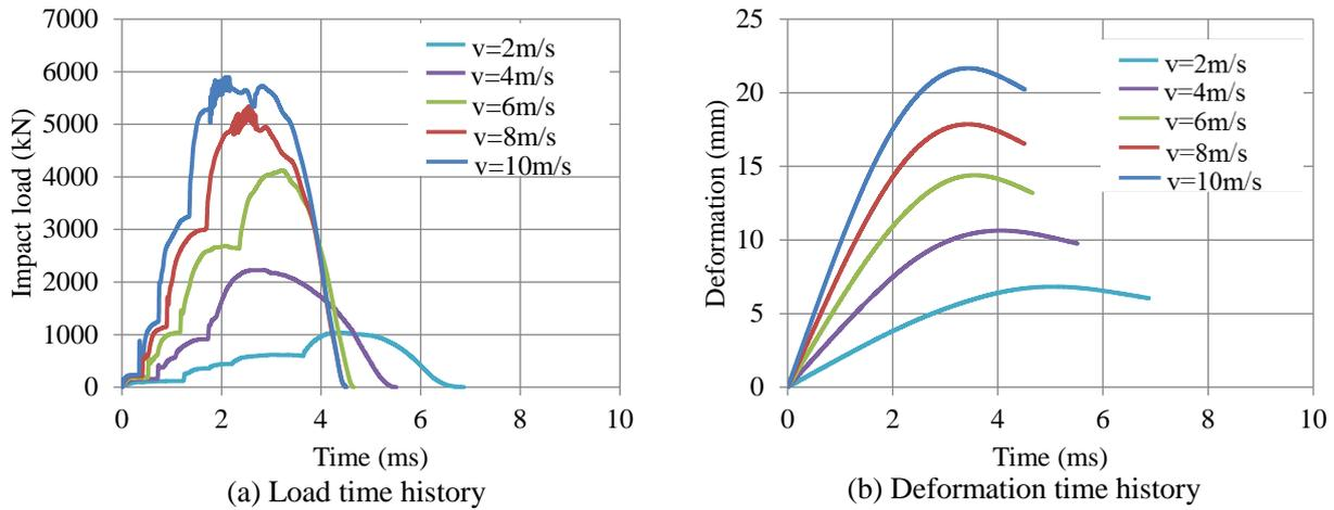
Figure 3 Concrete dam wing characteristics for an impacting rock with a diameter of 1m
