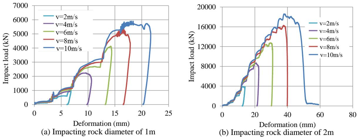
Figure 4 Impact load-deformation relation
