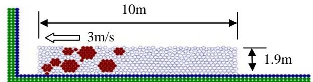
Figure 8 Debris flow model with rocks
