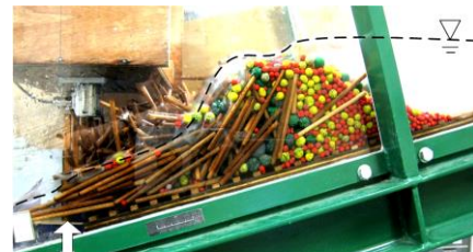
Dam (b) Volume 20% of wooden debris
