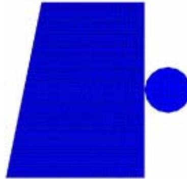
Fig.8 Concrete check dam wing under collision of rock (rock velocity  $V=10\text{m/s}$ , rock diameter  $D=1\text{m}$ )
