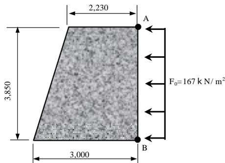
Fig.1 Concrete check dam wing under fluid force
