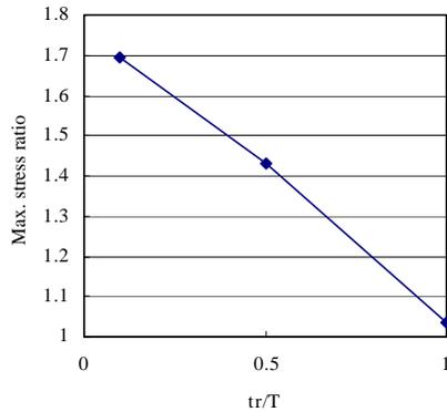
Fig.7 Max. stress ratio - rise time ratio relation
